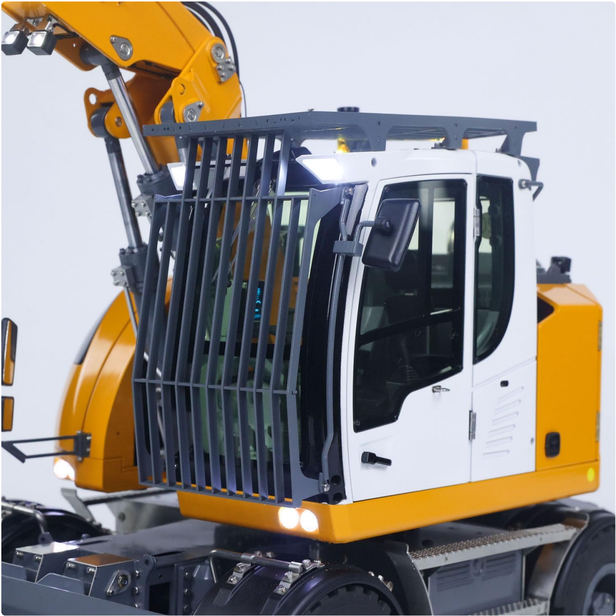
Figure 2: Detail of the excavator's cabin, showing the front guard rail and integrated spotlights.
