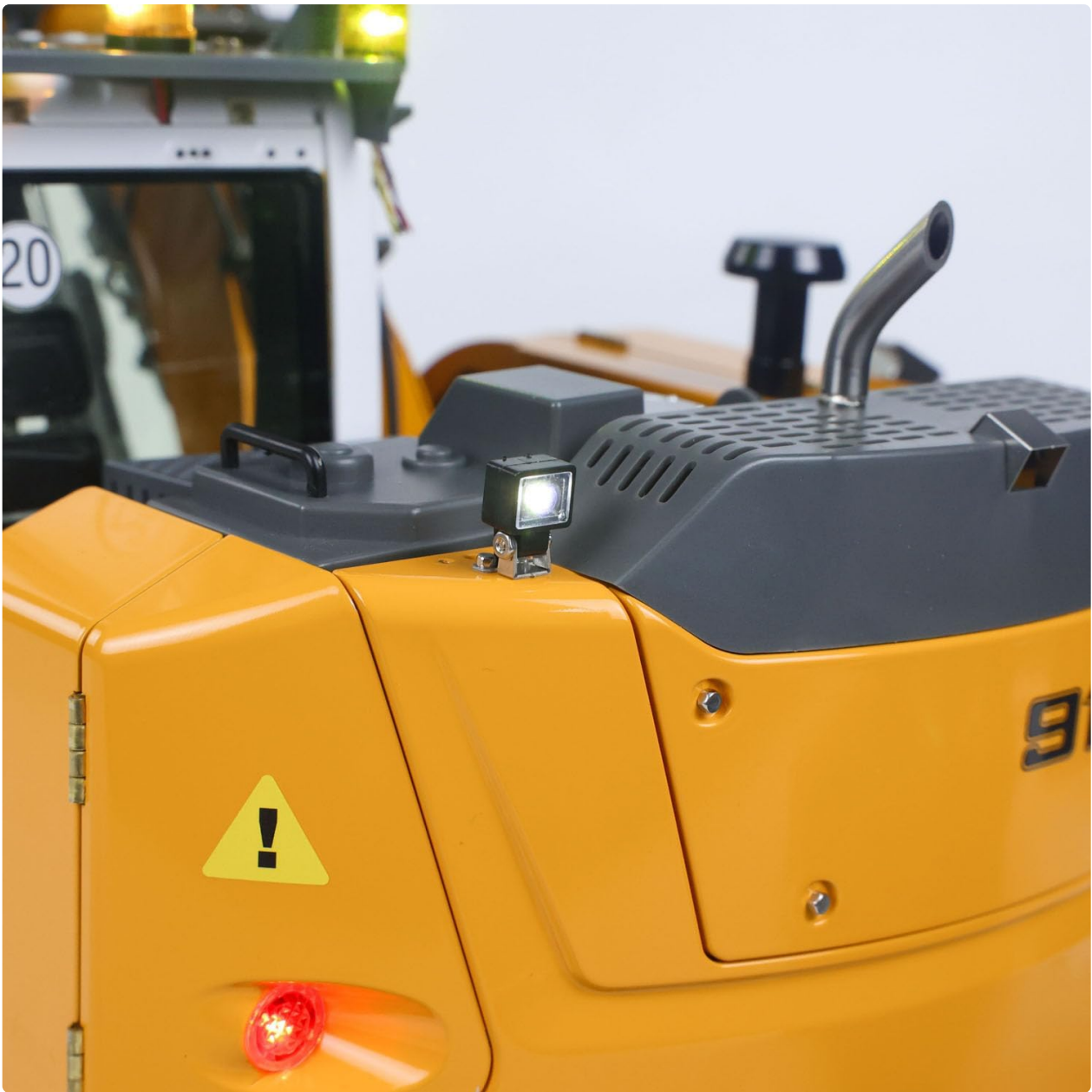
Figure 3: Rear view detail, highlighting a spotlight and a warning light on the excavator.
