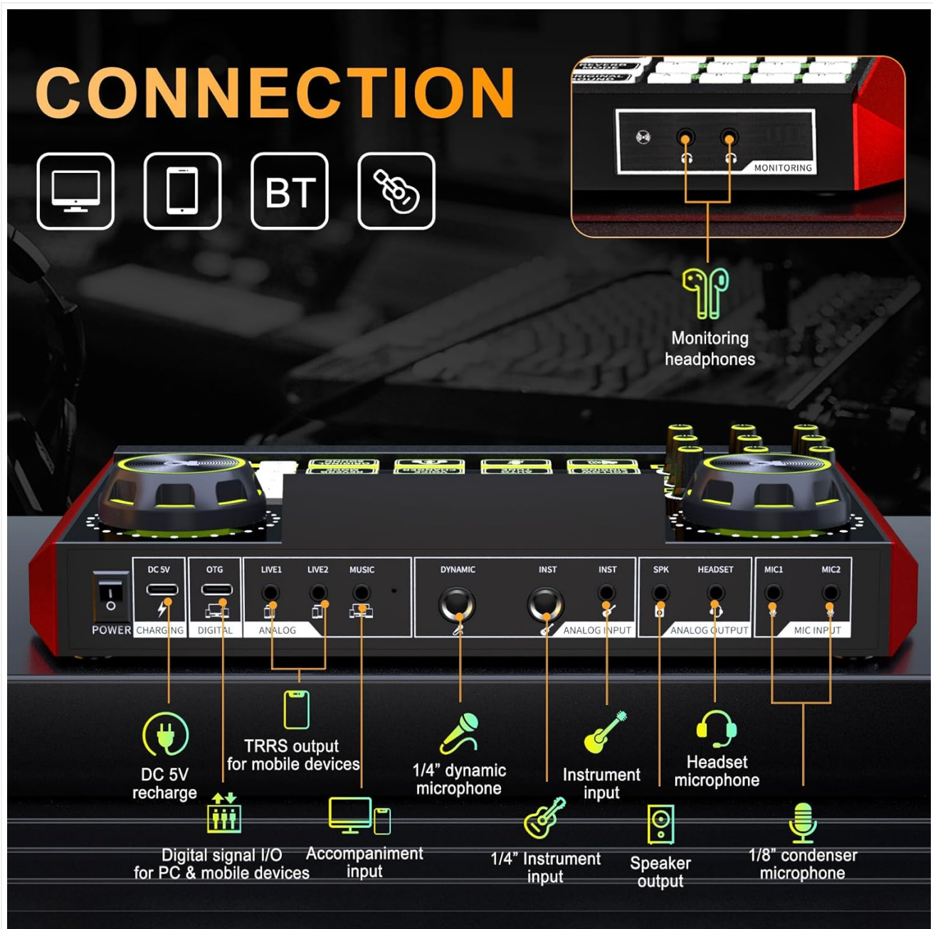
Figure 2: Overview of connection ports on the G9 mixer.
