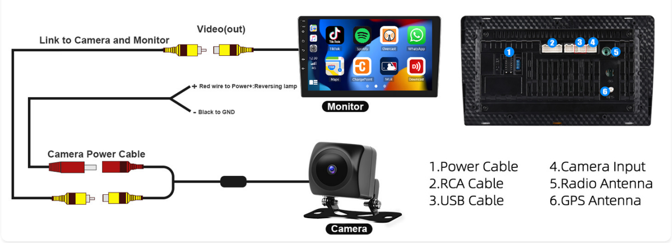
Image 2.2: Rear Camera Wiring Diagram.
