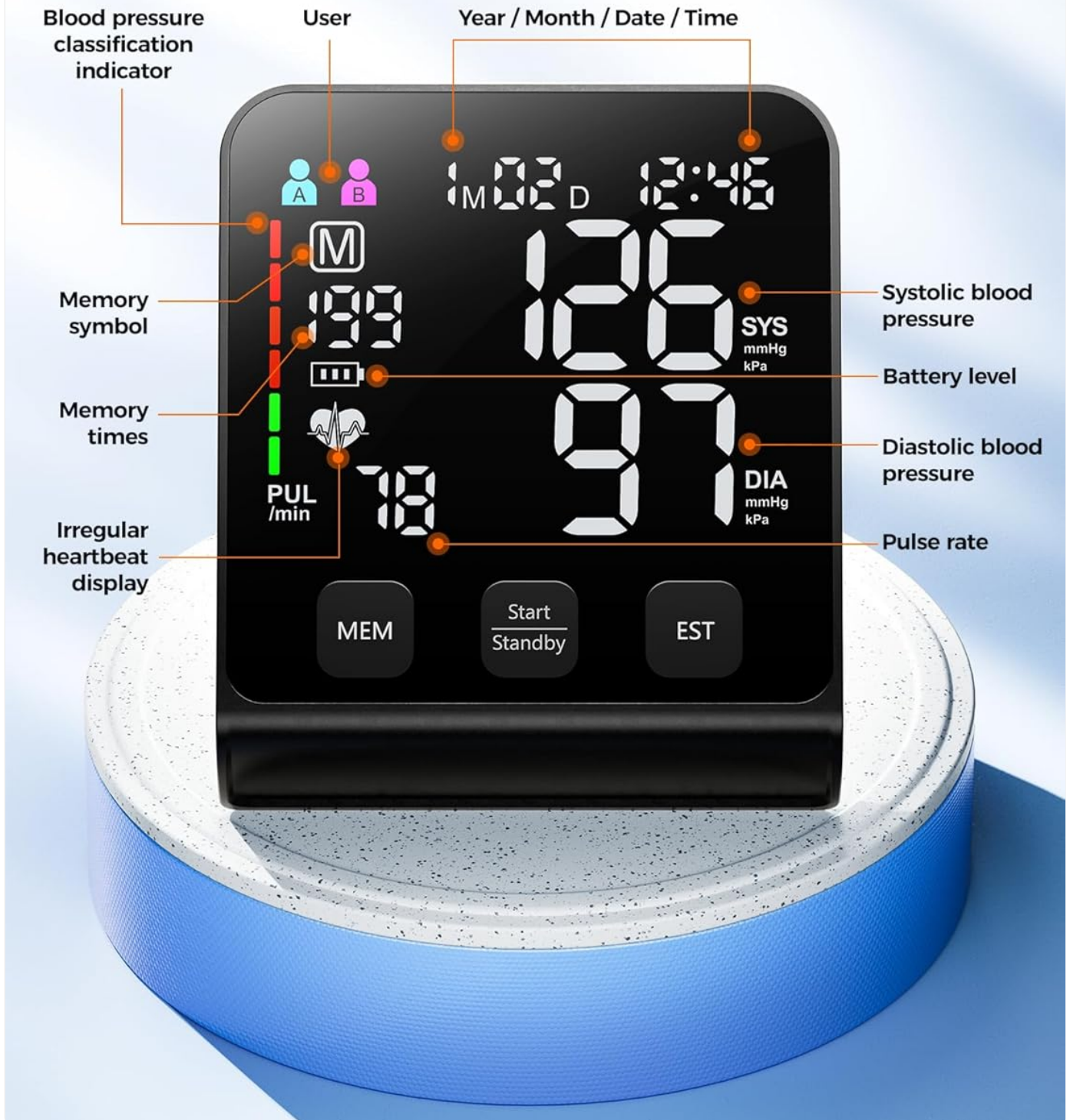
Image: A detailed diagram illustrating the various indicators on the monitor's LED display, including user selection (A/B), memory symbol, memory times, blood pressure classification indicator, irregular heartbeat display, pulse rate, systolic blood pressure, diastolic blood pressure, battery level, and date/time.
