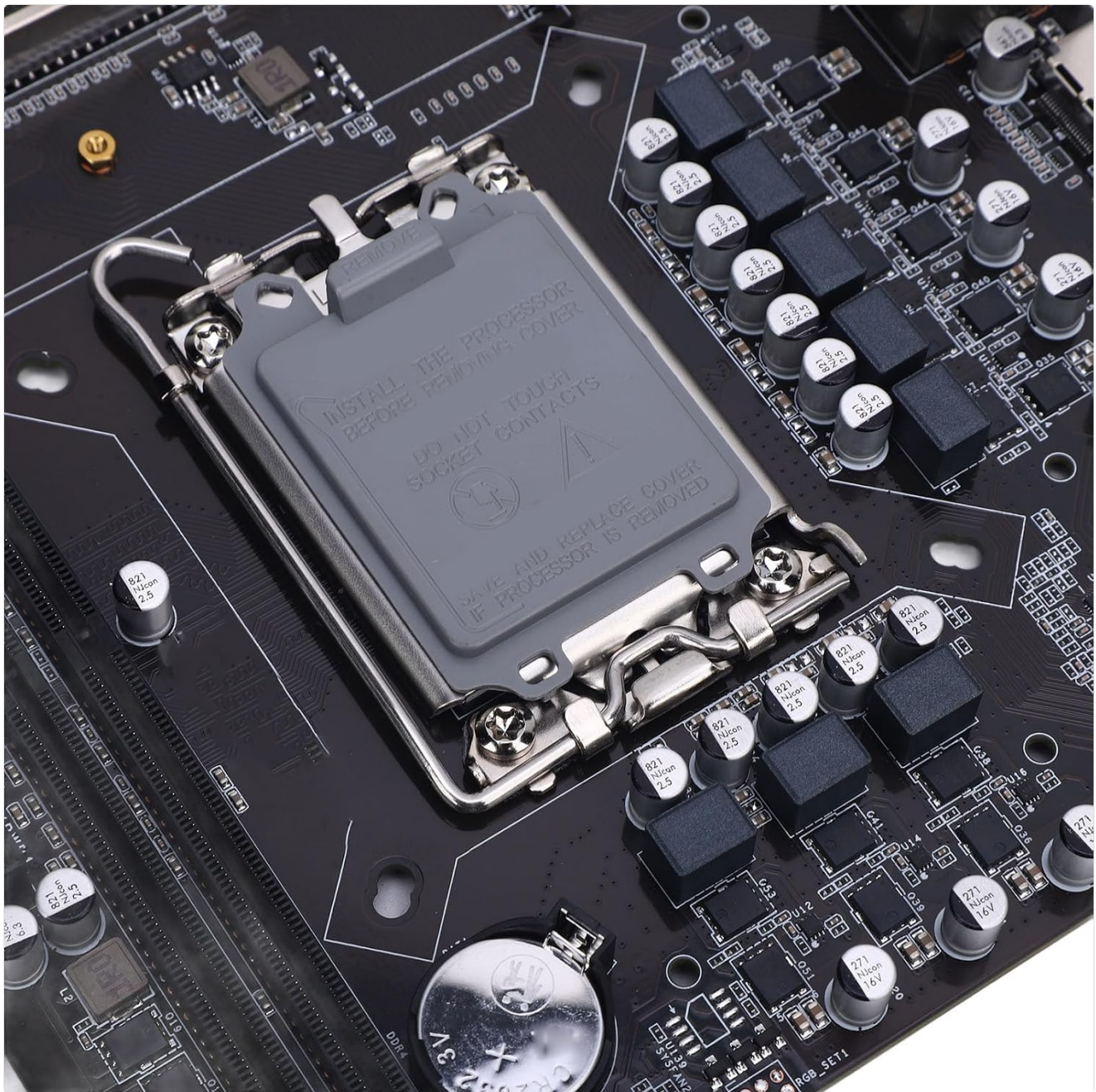
Figure 7: A detailed view of the CPU socket area, also showing the CR2032 CMOS battery located near the bottom right of the socket.
