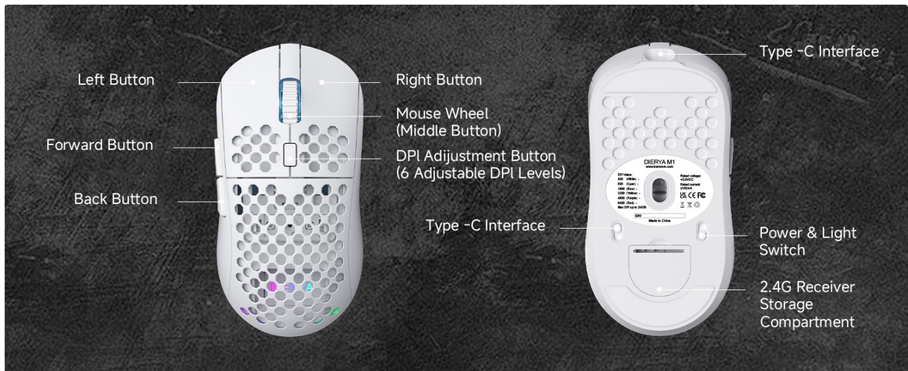
Figure 2: DIERYA M1 Mouse Components
