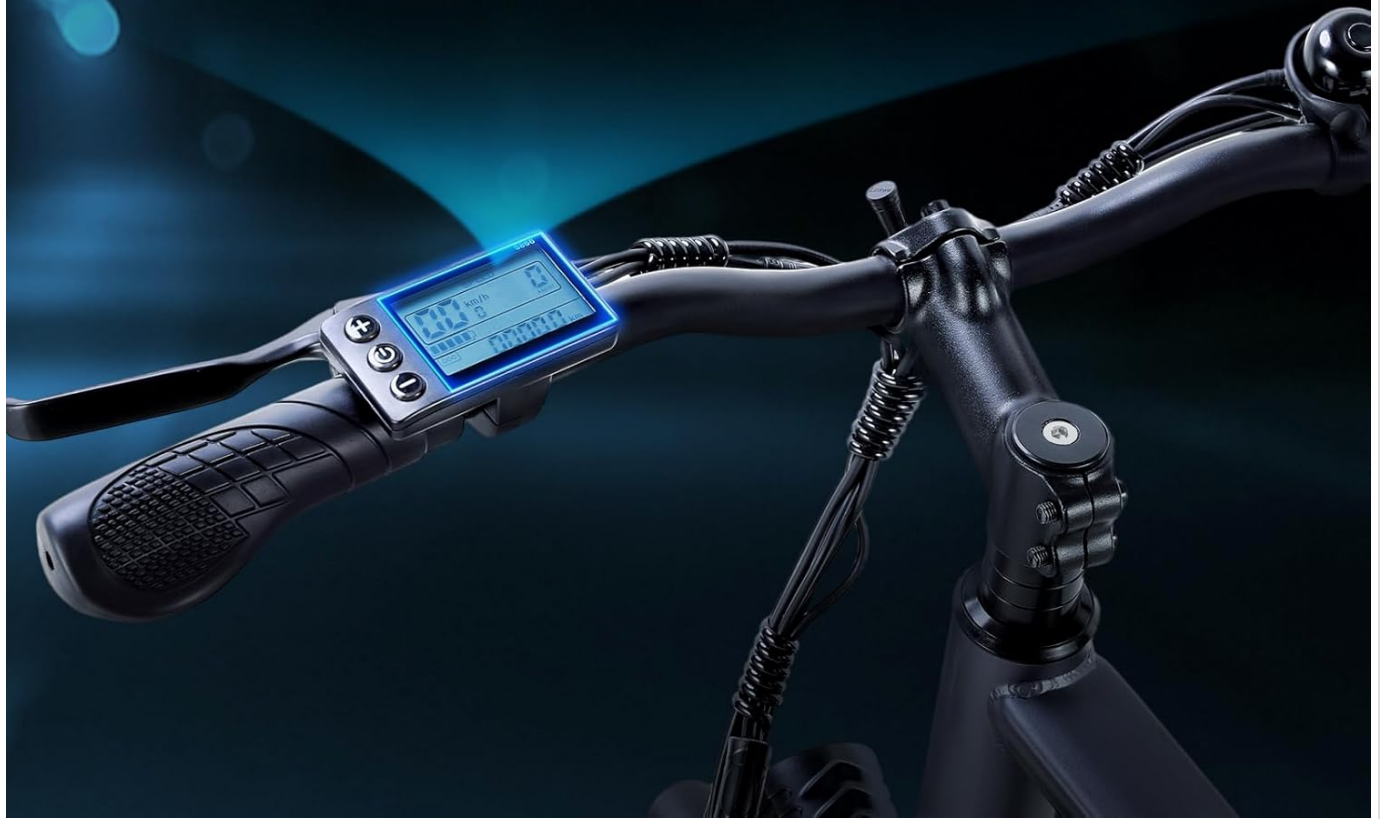
Image: Close-up of the TWOFISH Electric Bike's HD Smart LED Display, showing various indicators like assist level, speed, battery, light, odometer, error, and brake symbols.
