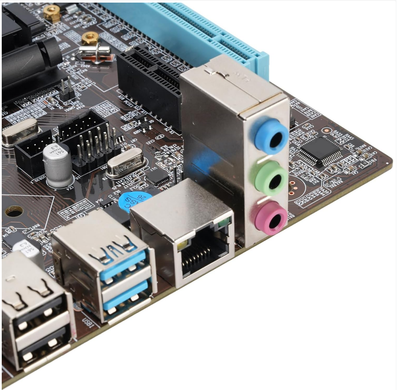
Image: Close-up view of the rear I/O panel of the ASHATA H110 motherboard, showing USB, VGA, HDMI, Ethernet, and audio ports.
