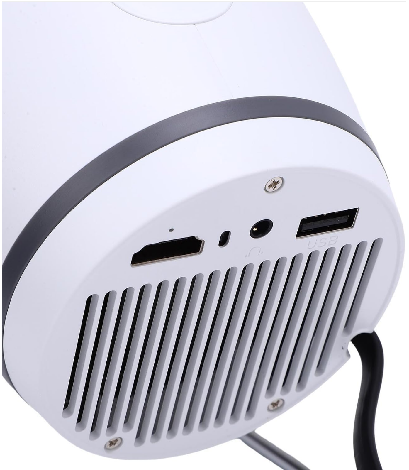
Figure 3.3: Rear view of the projector, displaying the various input and output ports including HDMI, audio out, and USB, along with ventilation grilles.
