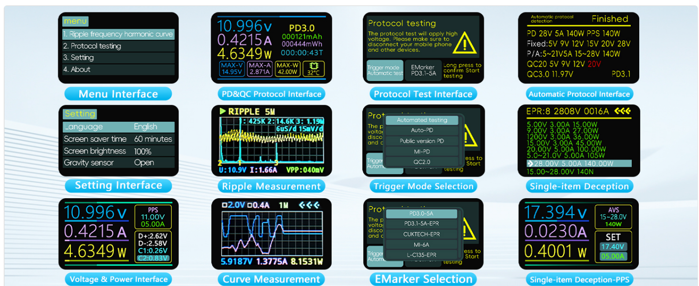
Figure 9: Overview of the various display interfaces, including the main menu, ripple measurement, protocol testing, settings, and detailed voltage and power readings, illustrating the tester's comprehensive data presentation.
