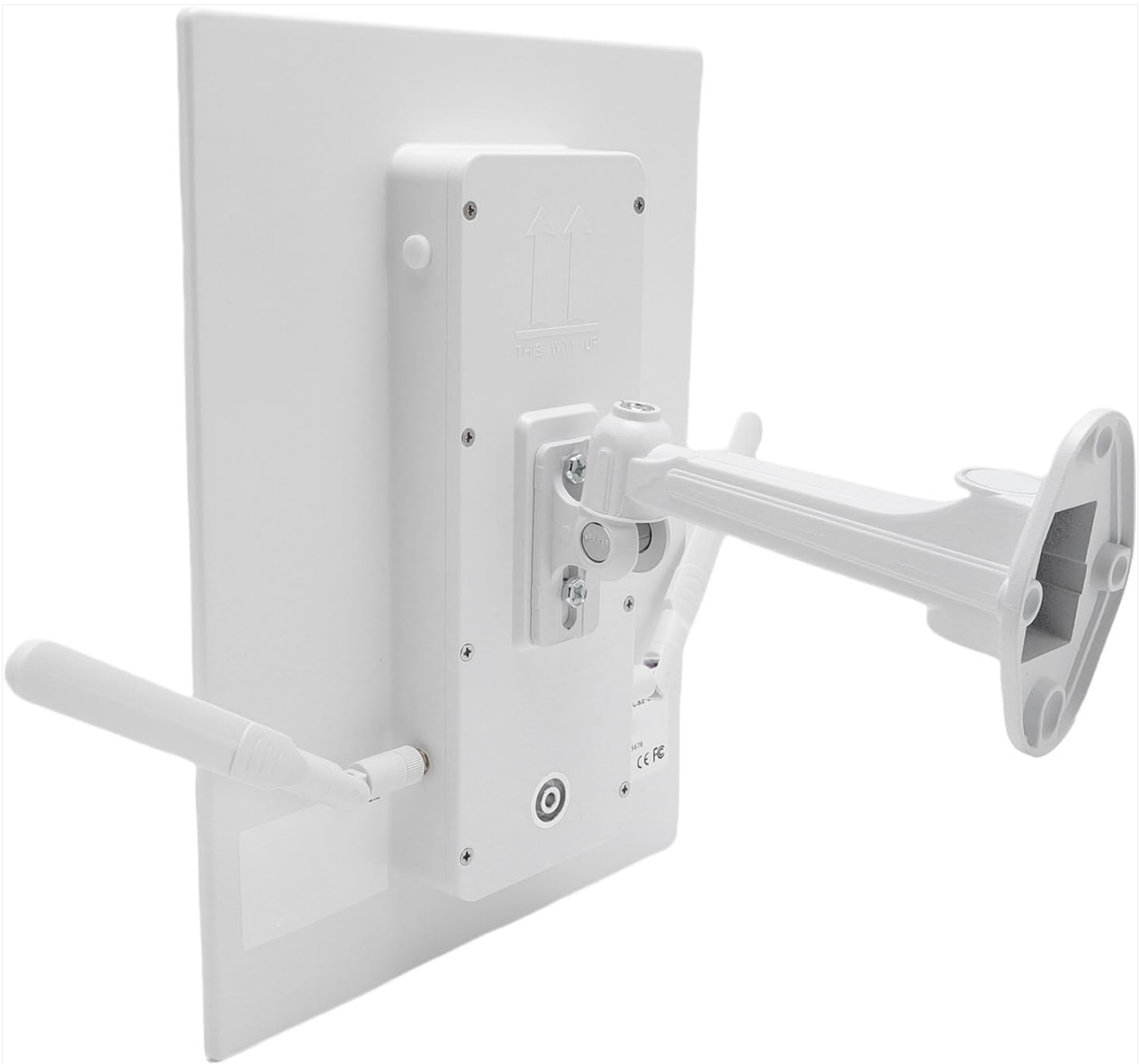
Image 3: Rear view of the router unit, highlighting the external antennas for WiFi and cellular connectivity.
