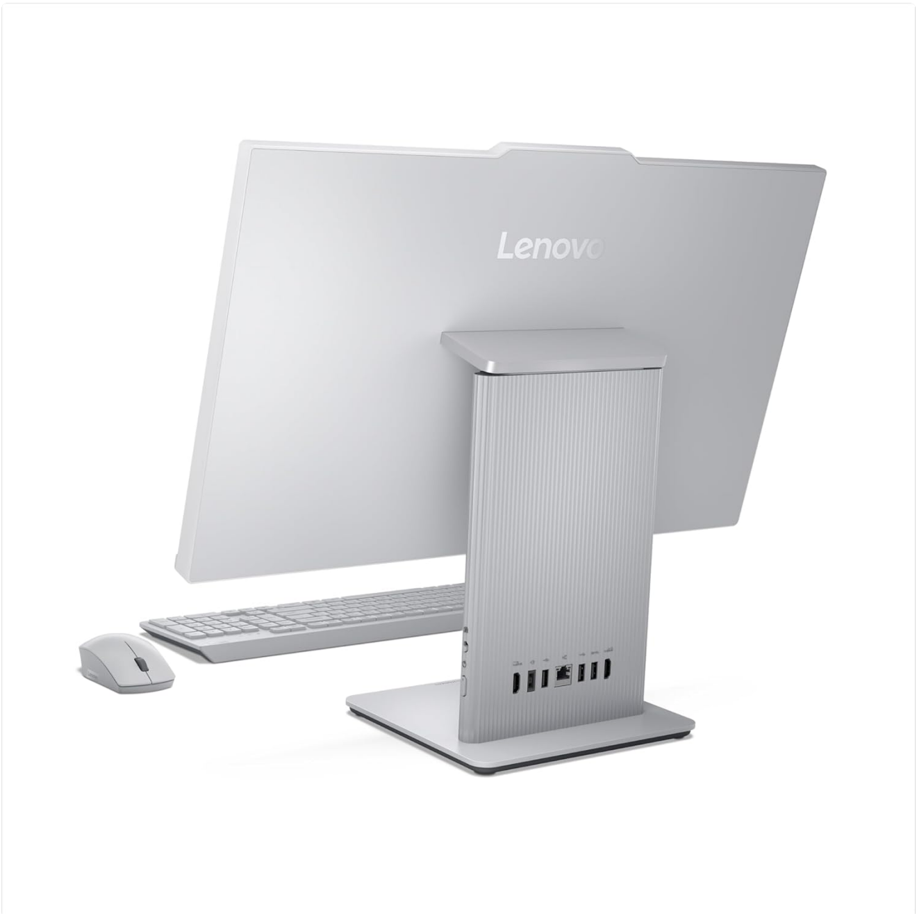
Image 3.2: The rear panel of the IdeaCentre AIO, detailing the available ports for power, USB devices, network, and external display connections.
