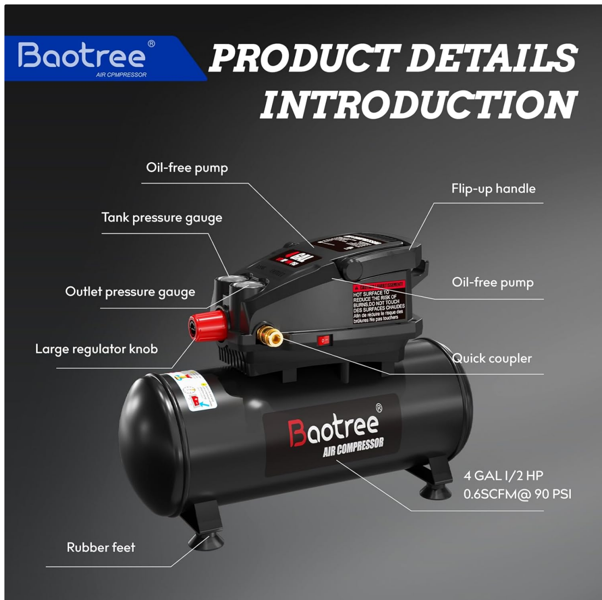
Image 3.1: Detailed view of the compressor's main parts.
