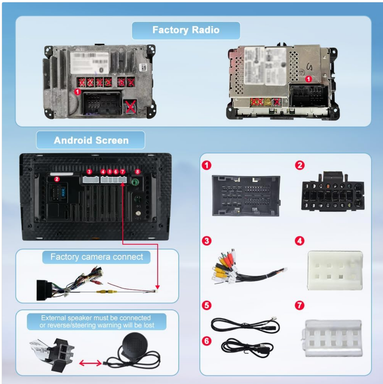
Image: All components included in the Junsun 2G+64G Car Stereo Radio package.
