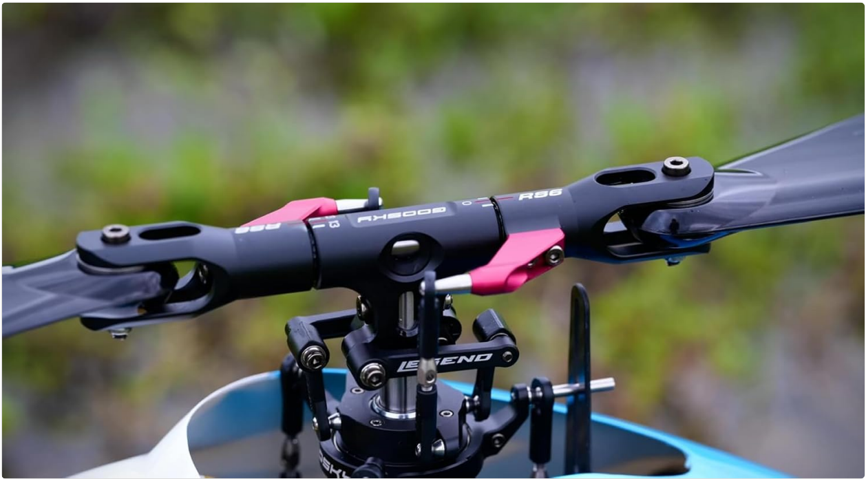
Image: Close-up view of the Goosky Legend RS6's full-metal main rotor head, highlighting its robust construction and pitch control arms.
