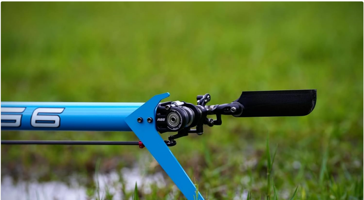
Image: Close-up view of the Goosky Legend RS6's tail rotor assembly, showing the tail blades and drive mechanism.
