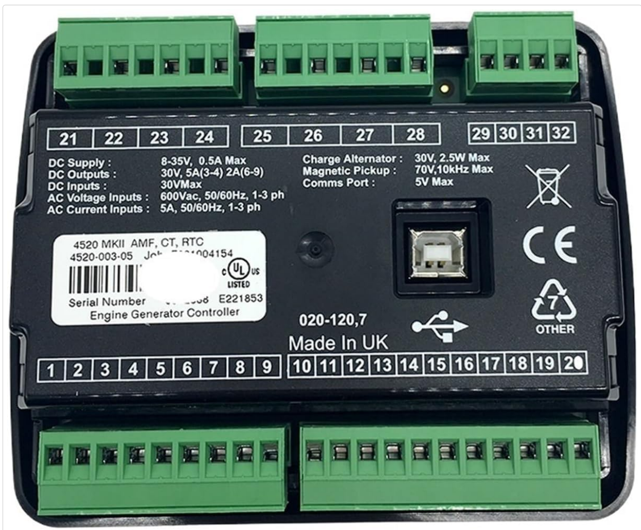
Image 4.2: A detailed close-up of the DSE4520 MKII's rear panel, showing the numbered terminal blocks and printed electrical specifications for DC supply, outputs, inputs, AC voltage/current, charge alternator, magnetic pickup, and comms port.
