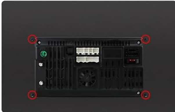
4 fixing holes for the machine
