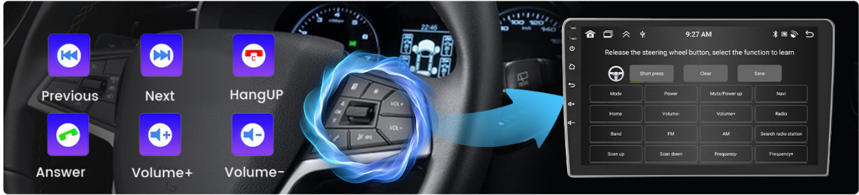
Figure 2.6: Interface for learning steering wheel controls, showing options to map functions like previous, next, hang up, answer, and volume.
