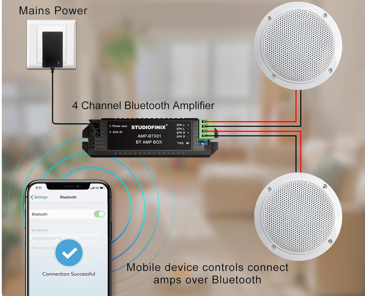
Image: Step-by-step wiring diagram for connecting speakers to the amplifier and power source.
