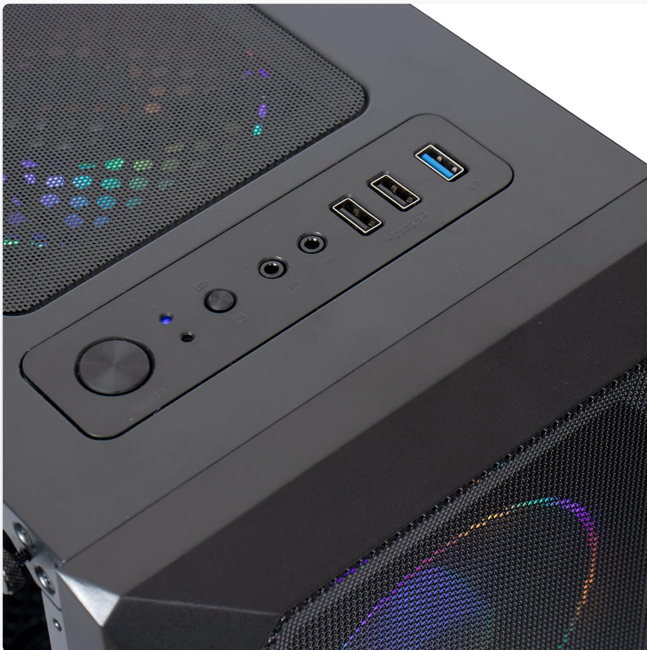
Figure 3: Top panel connectivity options including USB and audio ports.
