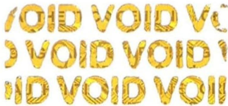
Figure 6: A sample of the unique serial tag and the 'VOID' pattern that appears if the warranty seal is tampered with or removed.
