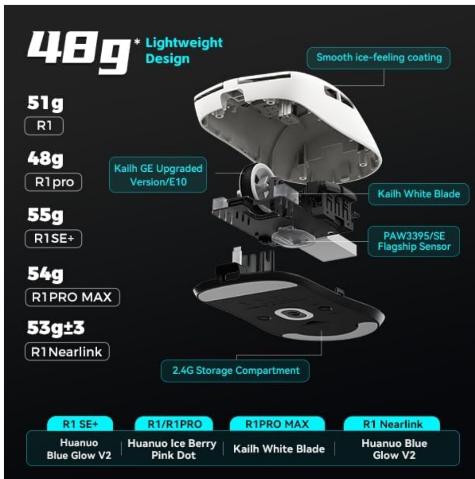
Image: Exploded view of the ATK VXE Dragonfly R1 mouse highlighting its lightweight internal components and showing weight comparisons for different R1 series models.
