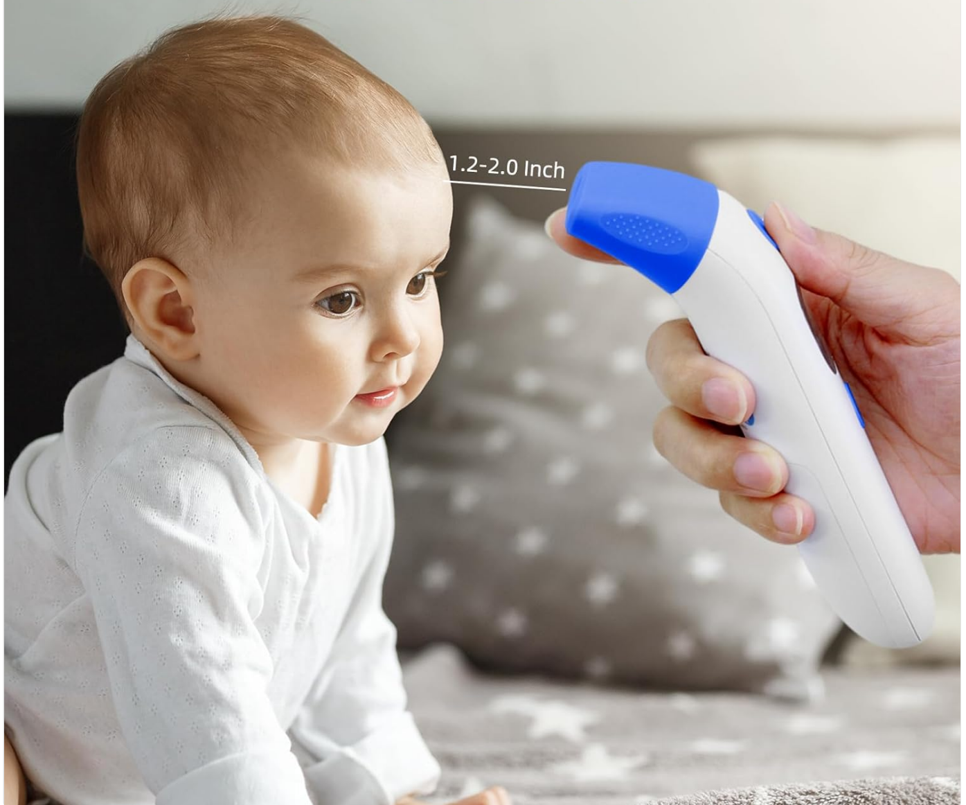
Figure 5: Taking a non-contact forehead temperature measurement.
