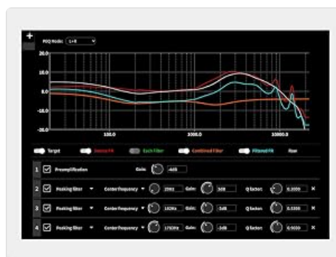
Image: The graphical interface for the 10-band PEQ, allowing detailed audio equalization.
