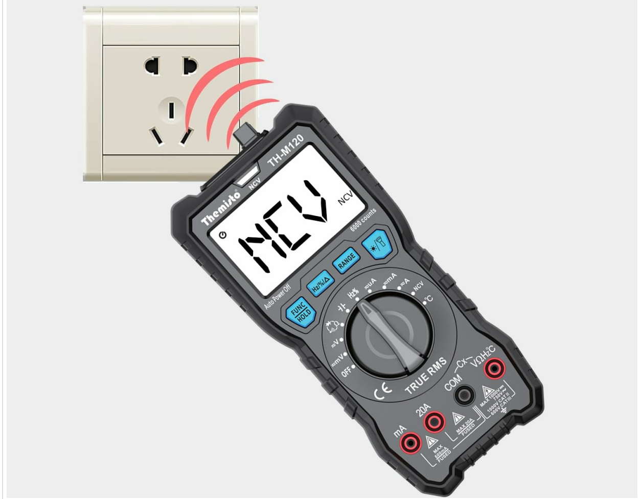
Figure 5.4: Using the NCV function to detect live wires safely.
