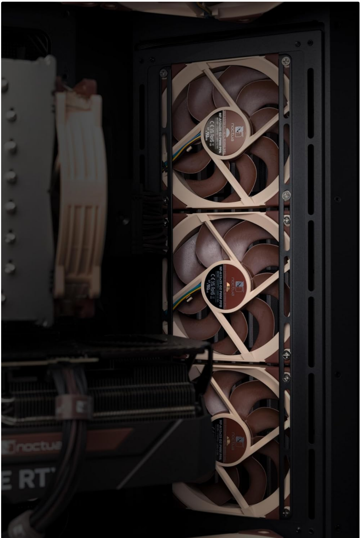
Image 4.1: Close-up view of the fan blades, highlighting the Progressive Bend impeller design for enhanced airflow.
