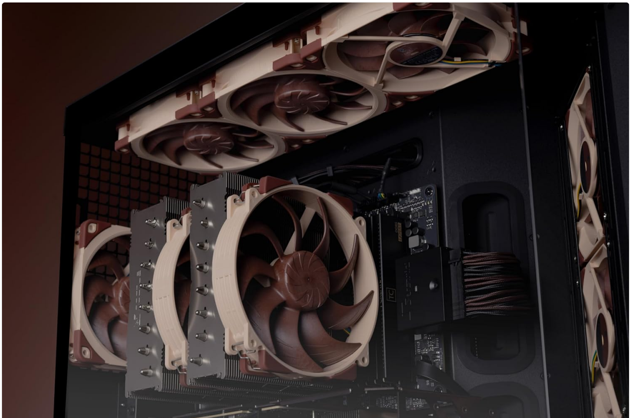
Image 3.2: Noctua fans mounted on a CPU cooler in a push-pull configuration, enhancing cooling performance.
