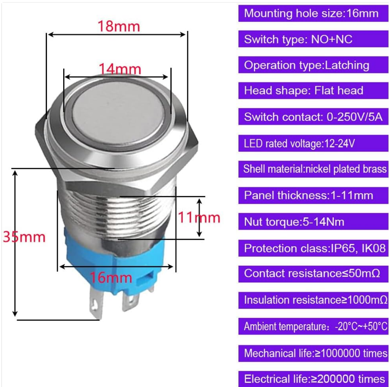
Image 3.1: Detailed specifications and dimensions of the Gebildet 16mm push button switch, including mounting hole size, switch type, and material.
