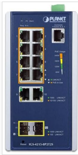
Figure 2.2: Front panel of the IGS-4215-8P2T2S switch. This view highlights the eight PoE+ RJ45 ports (1-8), two standard RJ45 ports (9-10), two SFP slots (11-12), console port, reset button, and LED indicators for power, alarm, link/activity, and PoE usage.
