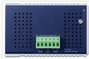
Figure 2.3: Rear panel of the IGS-4215-8P2T2S switch, showing the DC power input terminal block and fault alarm loading connections. The power input supports 48-54V DC, 6A max.
