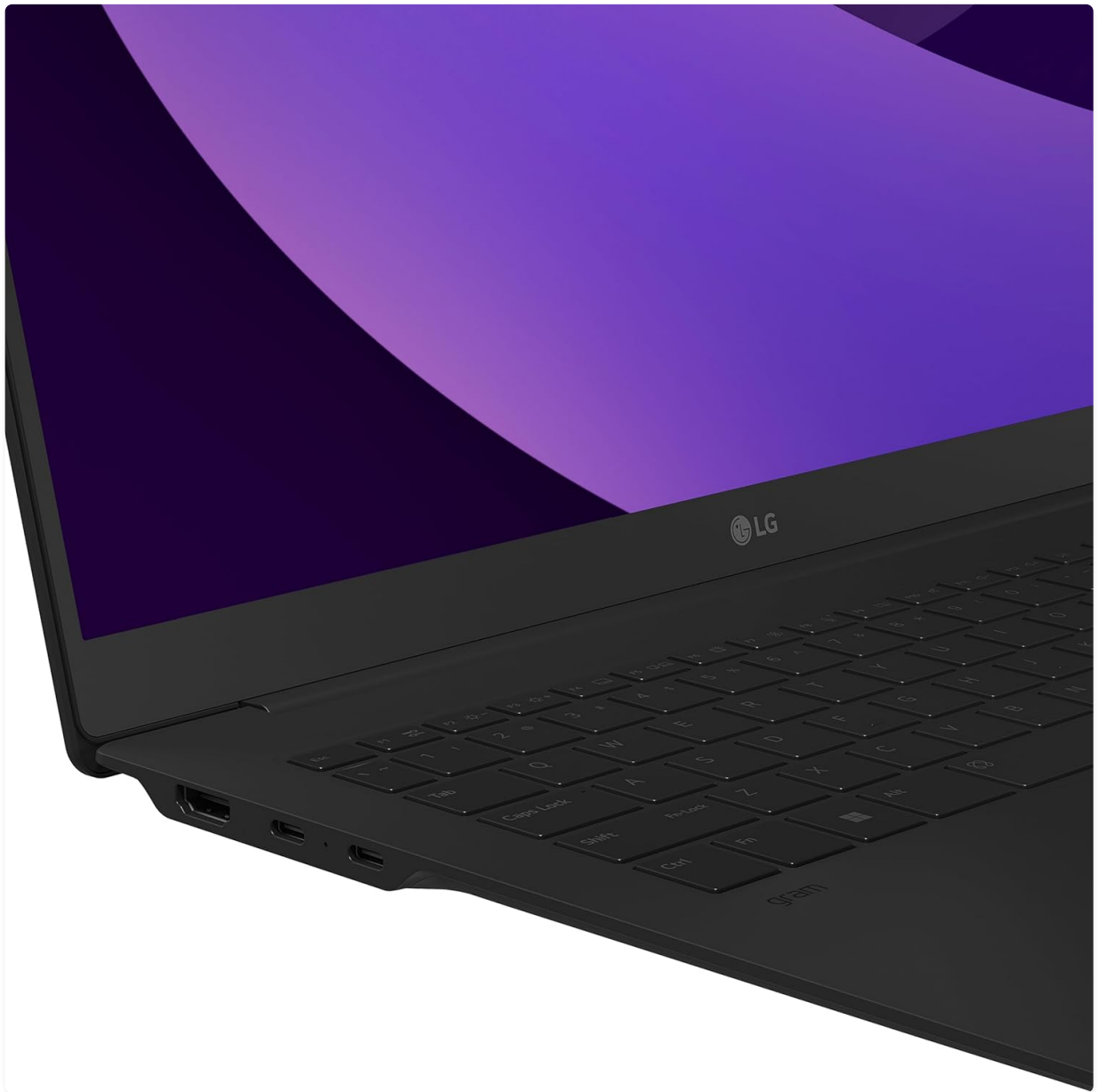
Figure 3.2: Left Side Ports. Includes USB 3.2 ports and a headphone/microphone combo jack.
