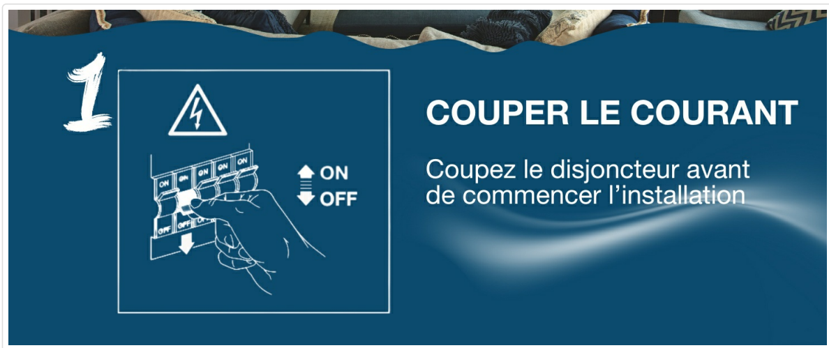
Image: Step 1: Disconnect power at the circuit breaker.
