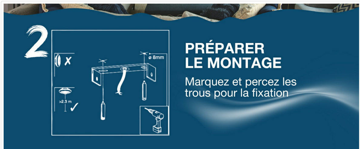
Image: Step 2: Mark and drill holes for the mounting bracket.
