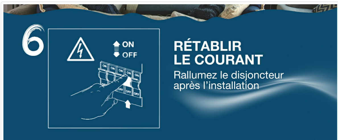
Image: Step 6: Restore power after installation.
