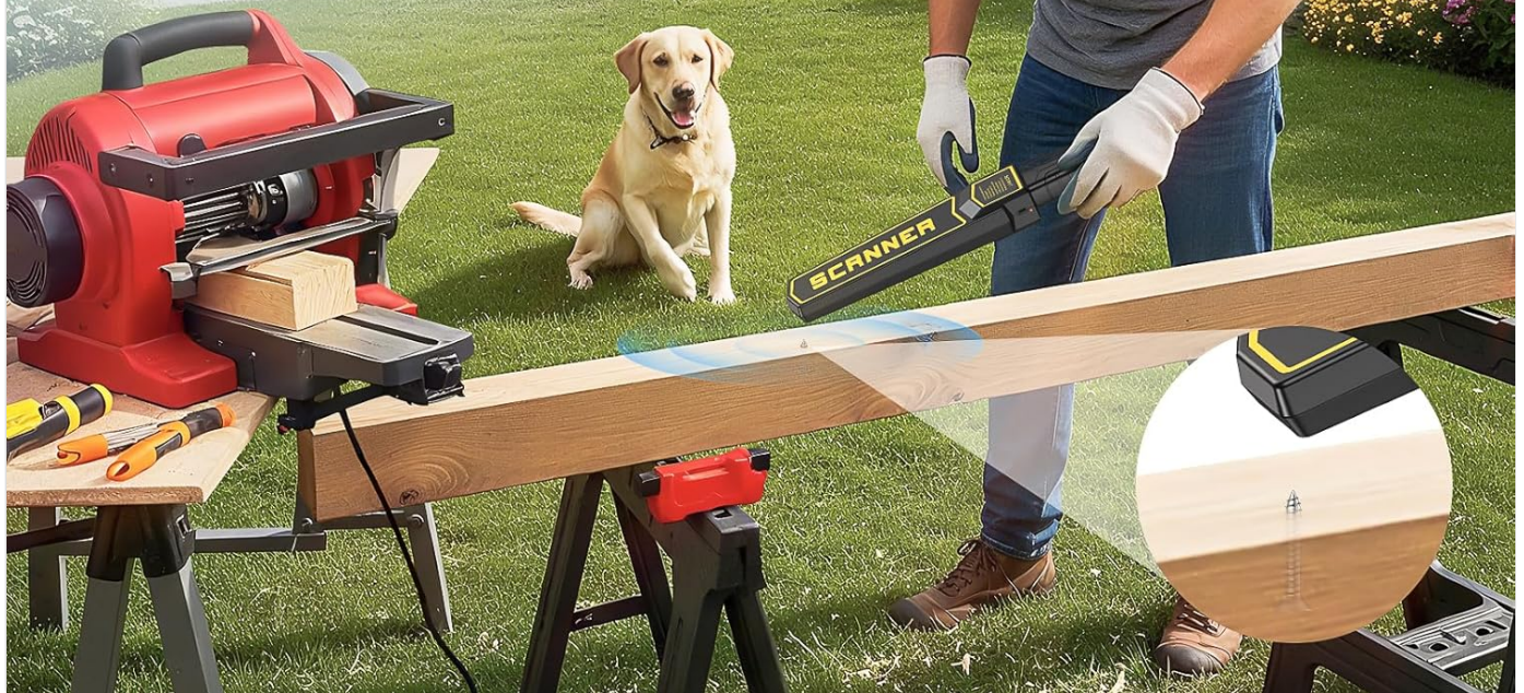
Image 6: A man is shown using the metal detector wand to scan a wooden beam, illustrating its application in woodworking to detect hidden nails and prevent damage to tools.
