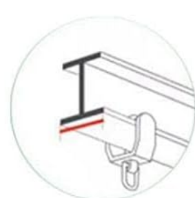
I-shaped track Bottom width 5-40mm Bottom ring width 0-5mm
