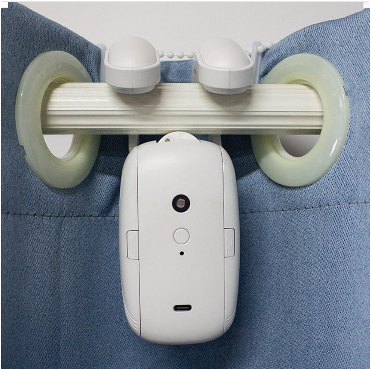
Image 4.1: The curtain opener installed on a Roman rod, demonstrating how it clips onto the rod.
