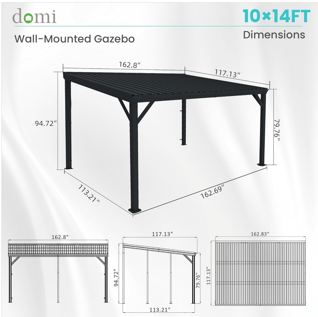
Figure 6: Detailed dimensions of the gazebo.
