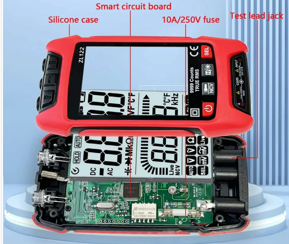
Figure 2: Internal Components and Safety Features
