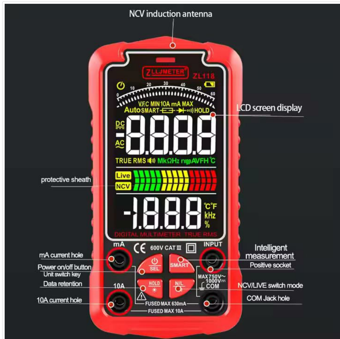
Figure 4.1: ZL118 Multimeter Components
