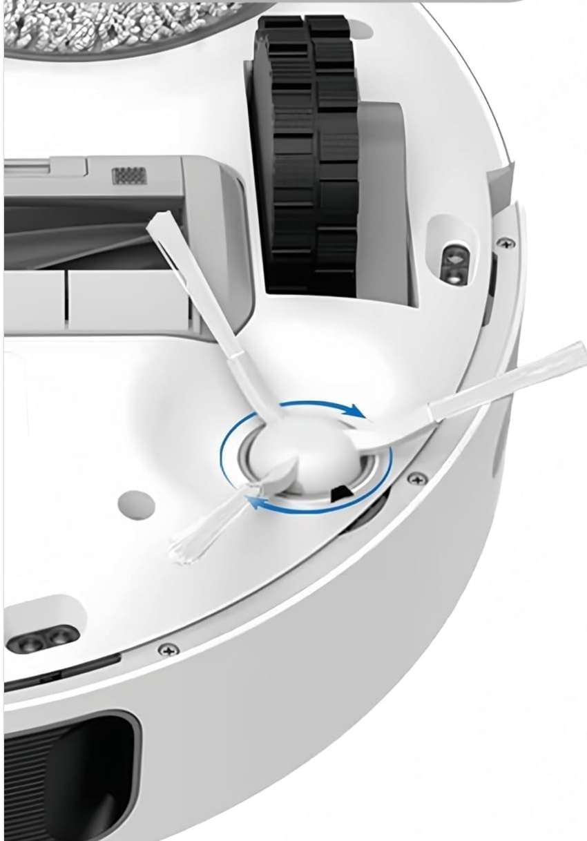
rotates with side bristle to prevent hairs from getting into structural gaps
