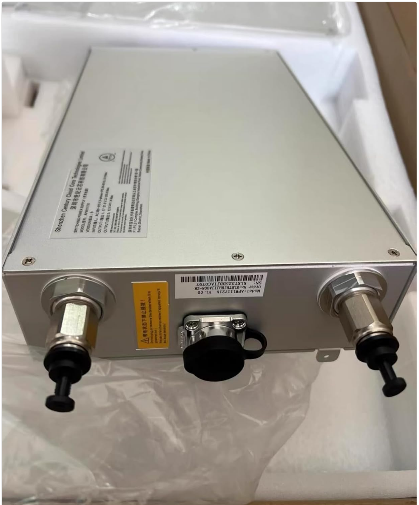
Figure 5.2: Detailed view of the APW11 Hydro Power Supply's connection panel, displaying the model number (APW11721C) and a warning label, indicating critical connection points and safety information.
