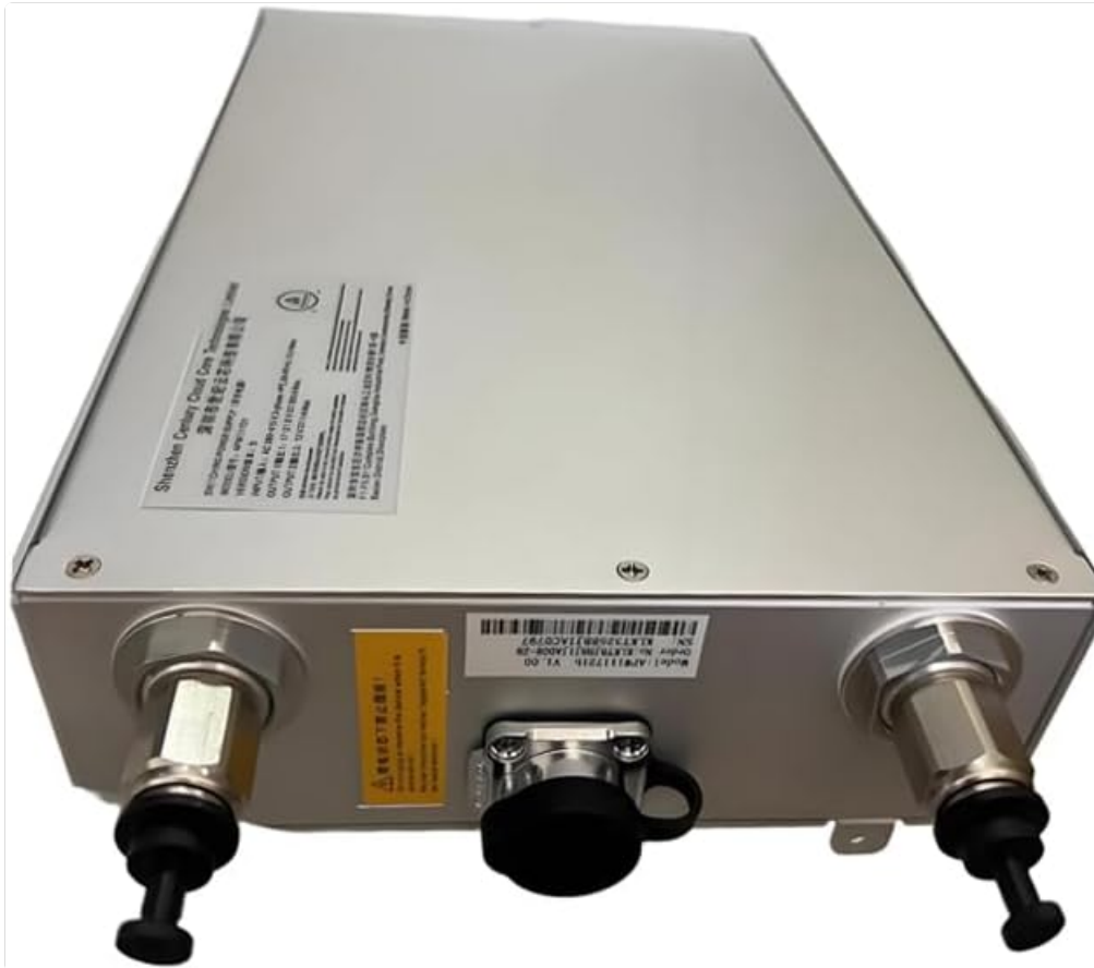
Figure 5.1: Top view of the APW11 Hydro Power Supply, highlighting the liquid cooling ports and power input connector. This view is crucial for understanding connection points.
