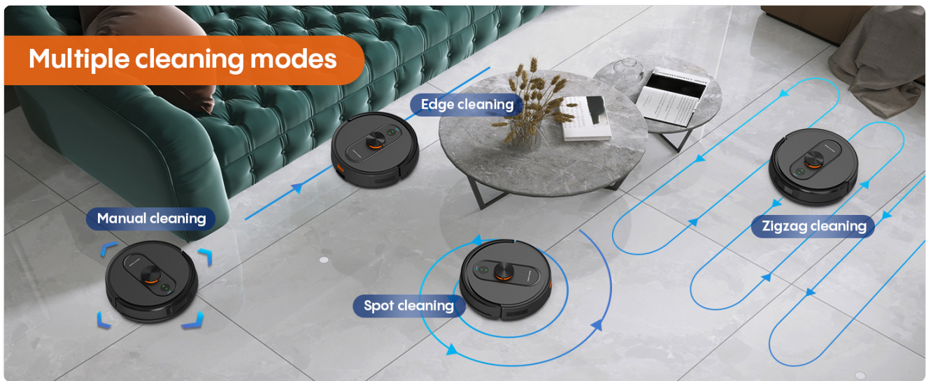
Figure 4.2: The robot supports various cleaning modes including manual, edge, spot, and zigzag cleaning patterns.
