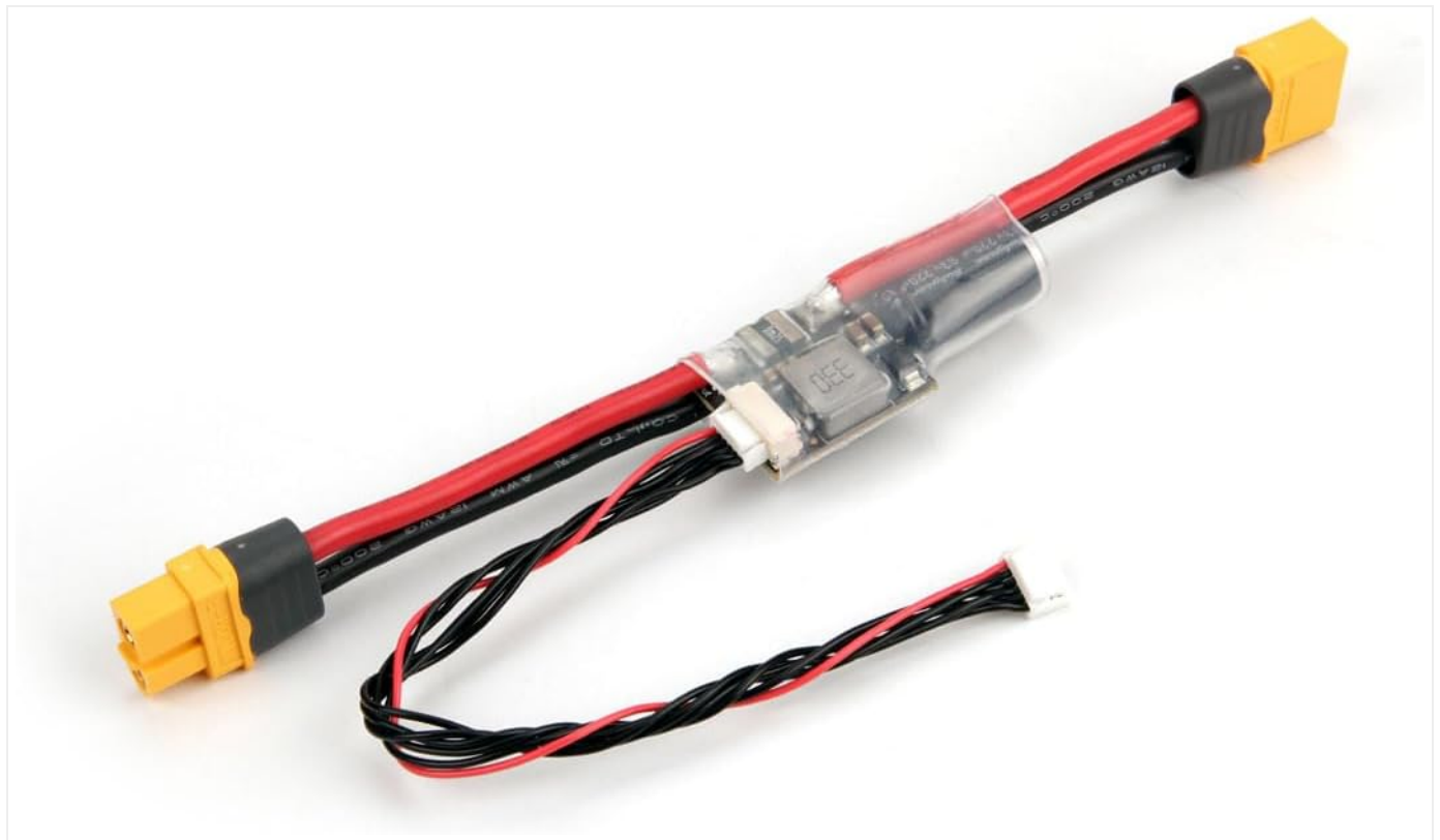
Figure 2: An example of a power module (PM02), used to supply power and monitor battery status.
