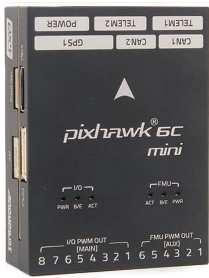
Figure 1: Pixhawk 6C Mini Flight Controller. This image displays the top surface of the flight controller, highlighting its various connection ports and PWM outputs.
