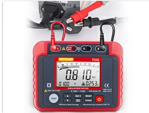
Figure 4.4: The megohmmeter connected to a power plug for an insulation resistance test.
