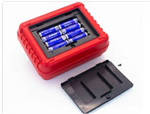
Figure 3.2: The battery compartment of the megohmmeter, showing the placement of AA batteries.
