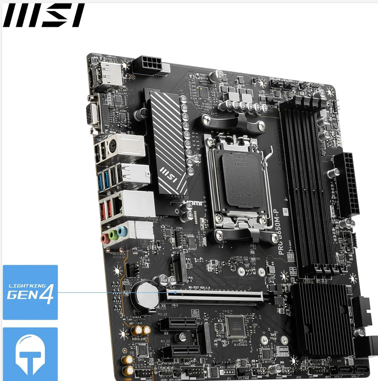
Figure 5.1: PCIe 4.0 x16 slot for graphics card installation.
