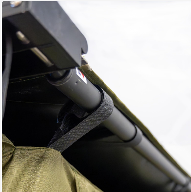
Image 3.1: Detail of the hook and loop strap securing the awning room to the main awning frame.
