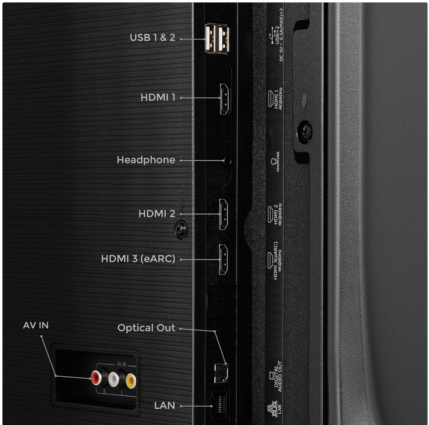
Image: Detailed view of the TV's connectivity panel. It shows 3 HDMI ports (one with eARC), 2 USB ports, a headphone jack, optical audio out, AV In, and a LAN port for wired internet connection.
