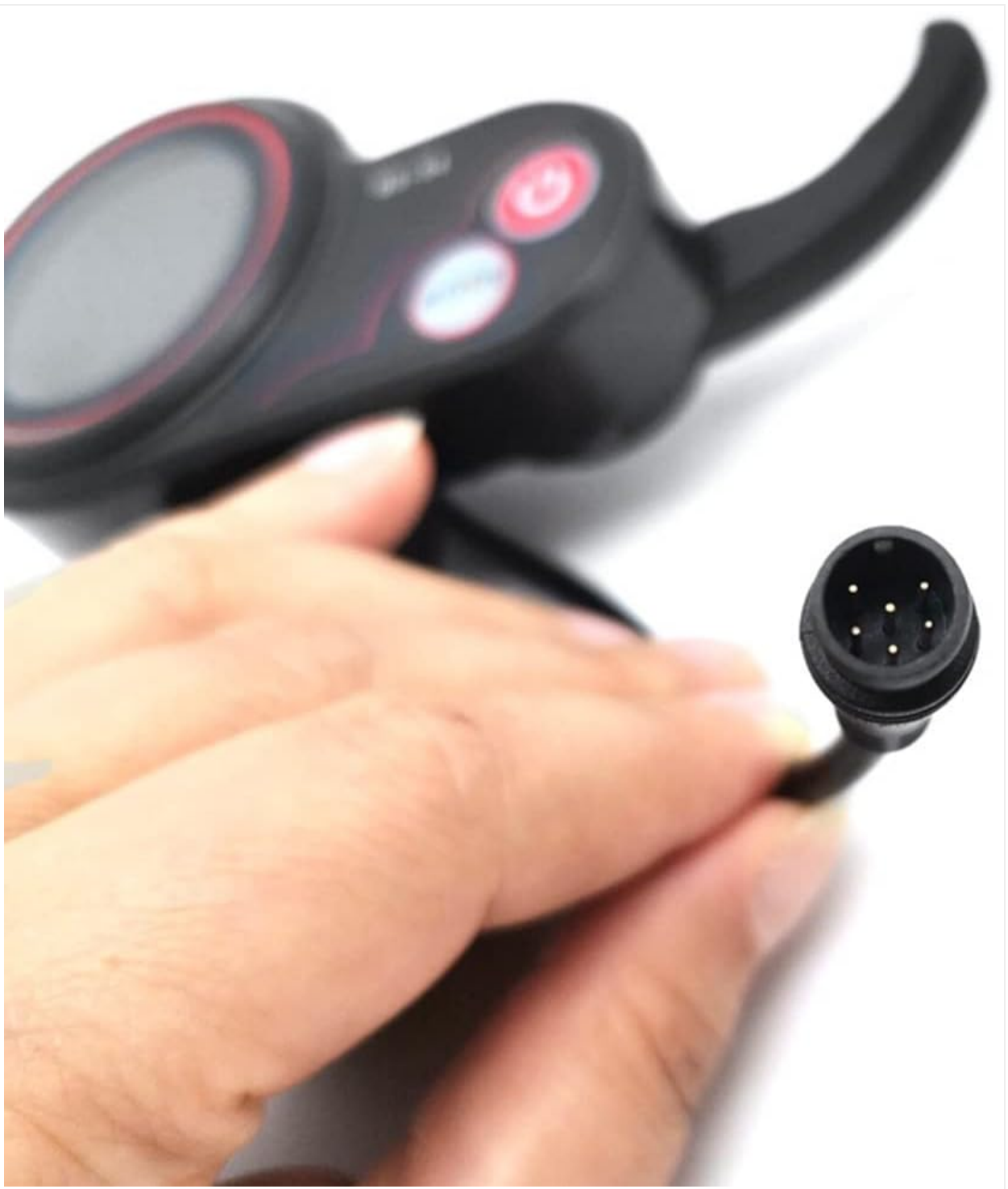
Figure 2.3: Close-up view of the 6-pin connector, which is used to connect the unit to the scooter's electrical system.
