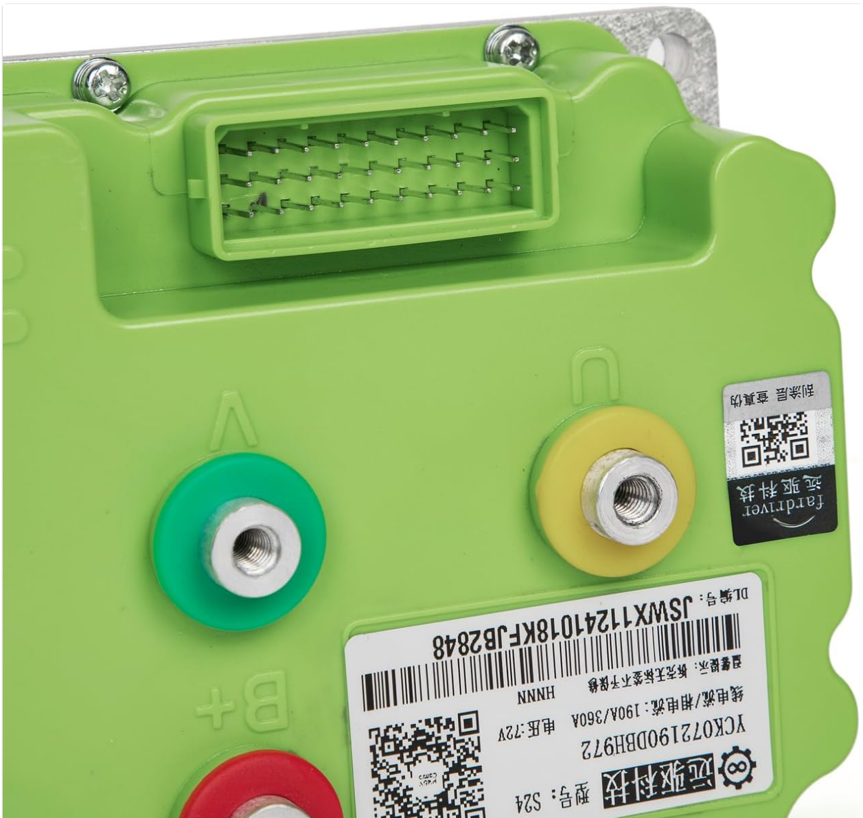
Figure 4: Detailed view of the controller's power and motor phase terminals, indicating the B+, B-, U, V, W connections with
