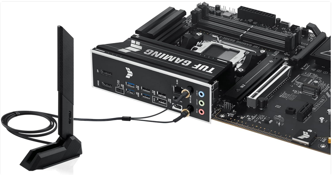
Figure 4.3: Wi-Fi antenna connected to the motherboard's rear I/O.
