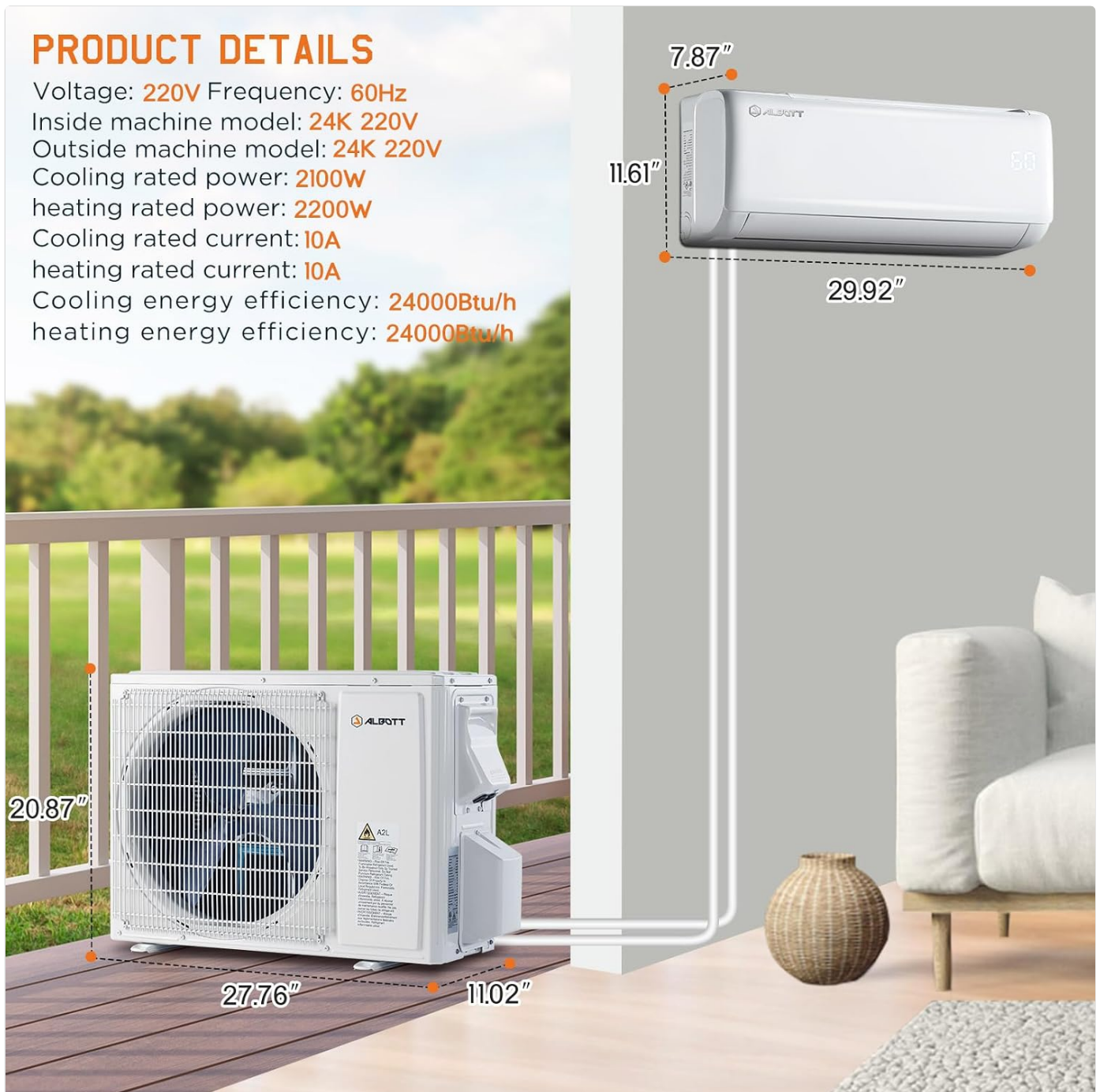
Figure 2: Product Dimensions. This image illustrates the dimensions of both the indoor and outdoor units, essential for planning installation space.
