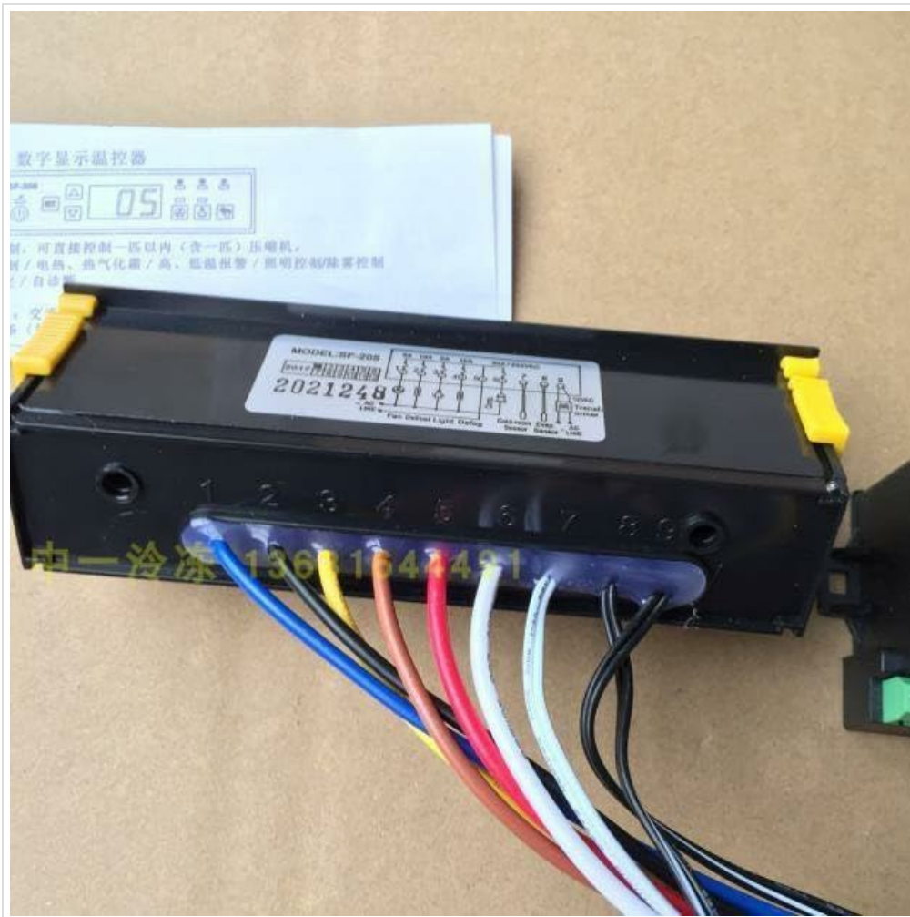
Image: The SF-205 main controller unit with various colored wires connected to its terminals. This view shows the overall physical structure of the device and its primary wiring points.
