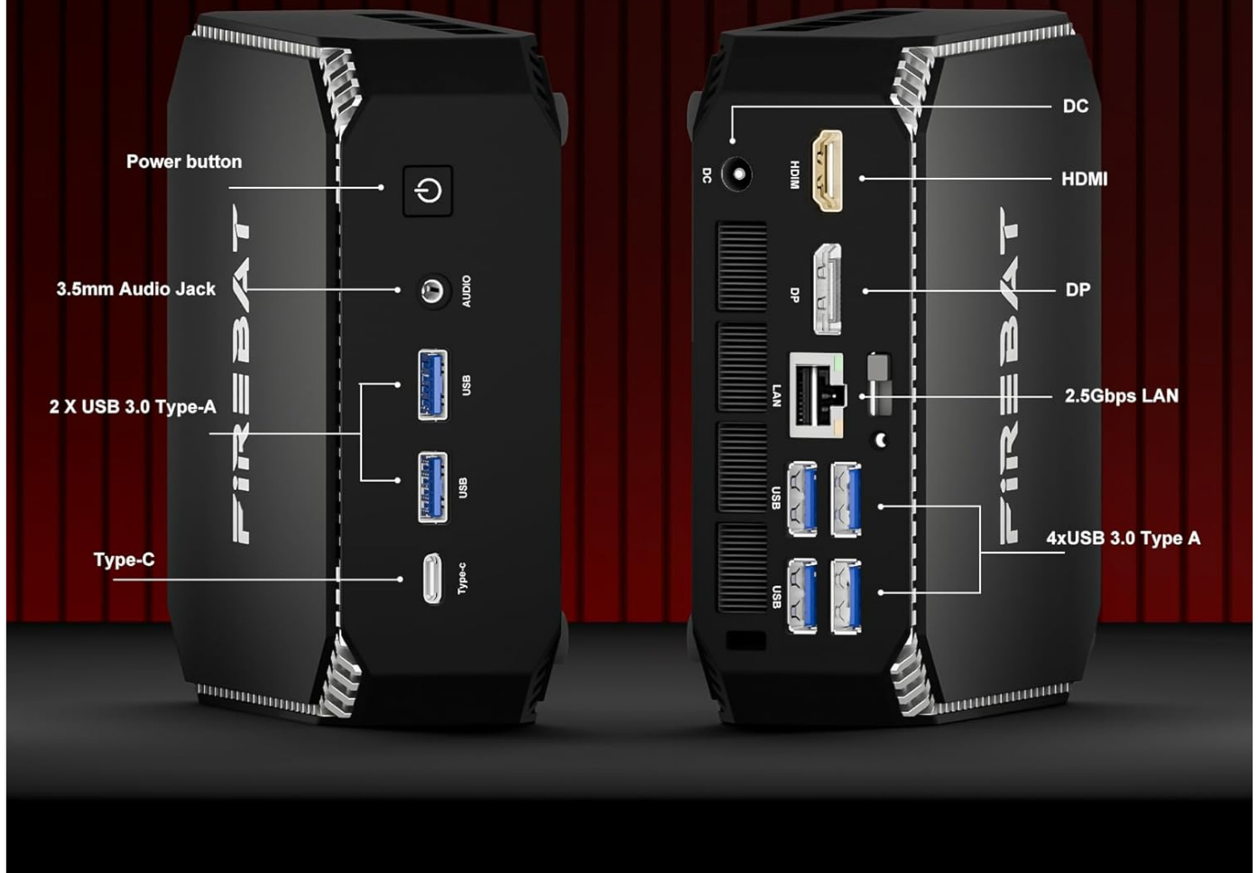
Figure 3.1: Overview of ports on the FIREBAT A6 Mini PC, including Power button, 3.5mm Audio Jack, USB 3.0 Type-A, Type-C, DC-IN, HDMI, DisplayPort, and 2.5Gbps LAN ports.
